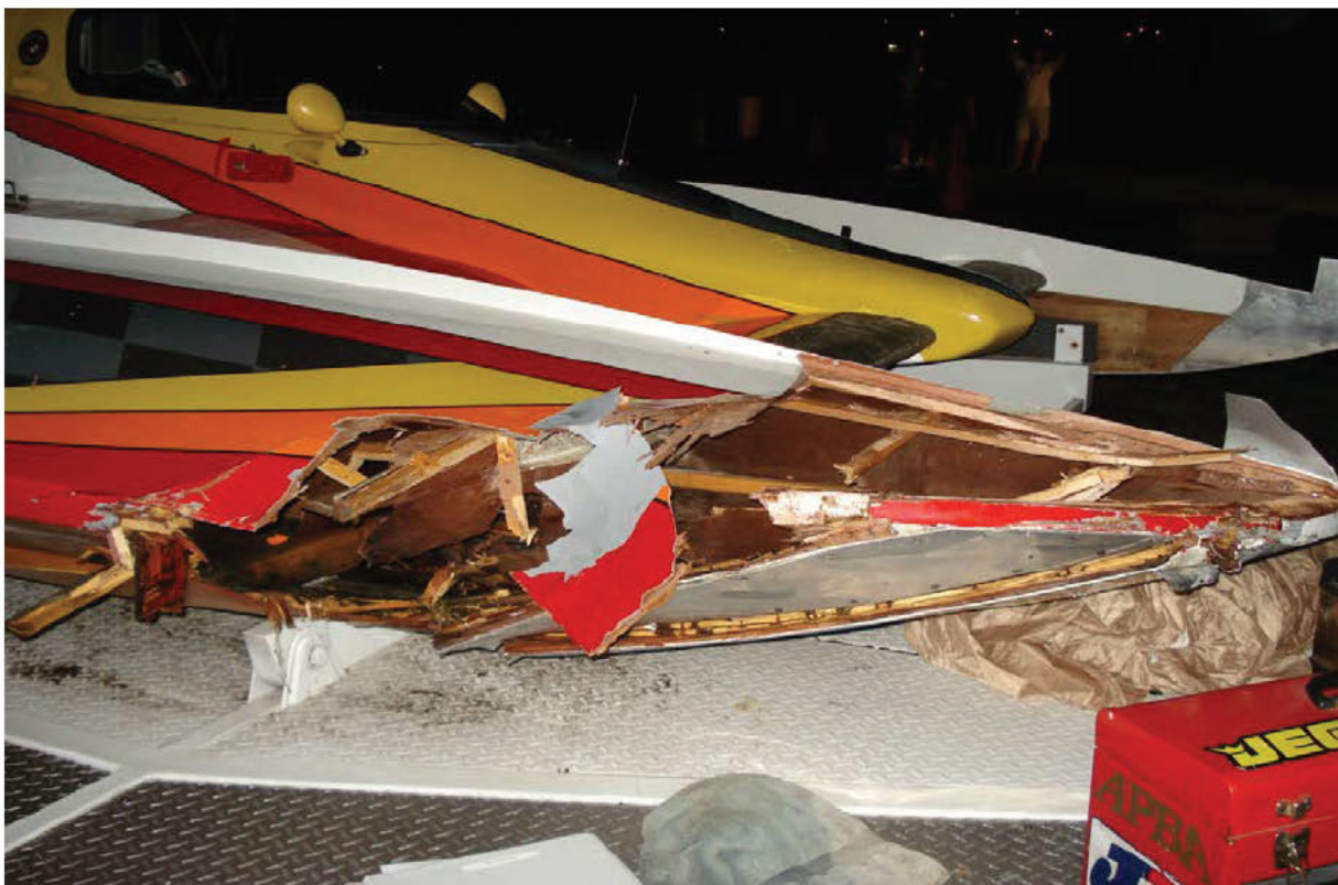
Figure 13.1 - Image of the extent of damage to starboard sponson of the GNH-12 taken the night of casualty.
