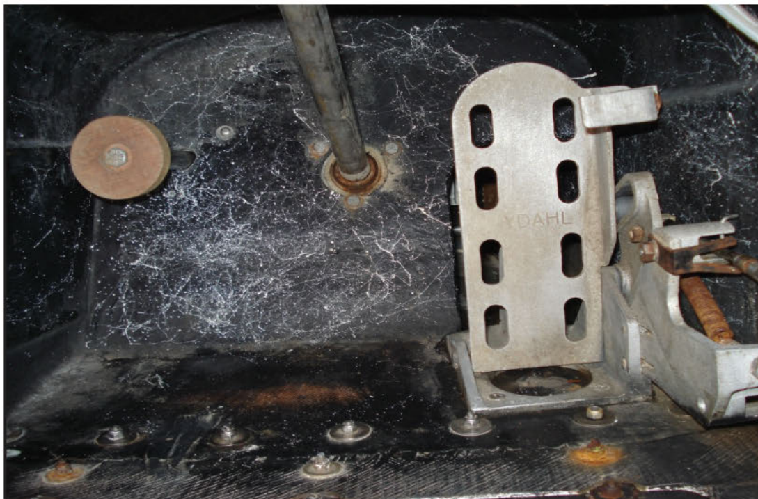
Figure 4.2- Image of the GNH-12's canard control (left) and accelerator (right)
